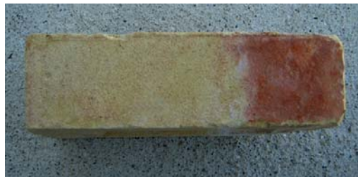
RED STAIN REMOVAL FROM YELLOW BRICK
